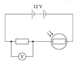
At a certain light intensity, the LDR has a resistance of 480  $\Omega$  and the voltmeter reading is 2.0  $V_{\cdot}$
