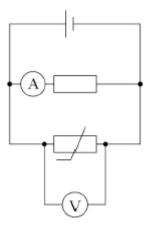
The temperature of the thermistor is increased.
