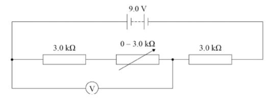
The resistance of the variable resistor is varied from 0 to 3.0  $k\Omega$ .
